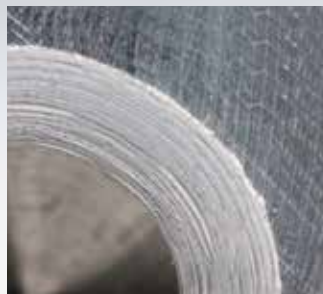
Countersinking with standard countersink
