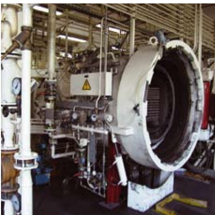
Efficient: Modern Sinter-HIP-furnaces in the carbide production.
