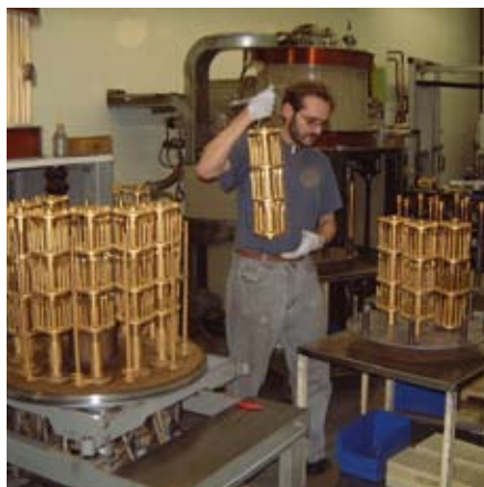
Know-how: The coating process for Guhring tools.
